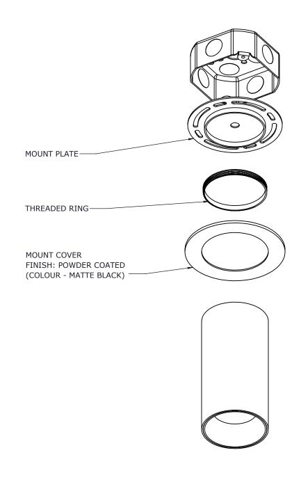
LAMPING: AC LED BOARD 7W, 700LM, 3000K, CRI 90 TRIAC DIMMING
